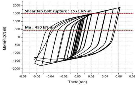
(a) Direct-welded flange connection
