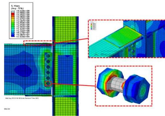
(b) Welded flange plate connection
