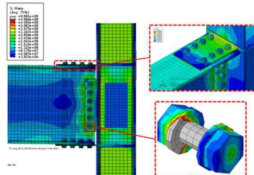
(c) High-strength bolted flange plate connection
