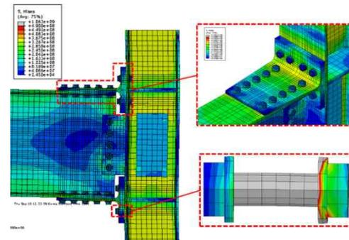
(d) High-strength bolted double split tee connection
