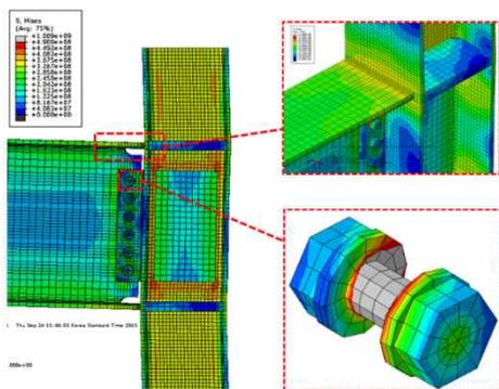
(a) Direct-welded flange connection
