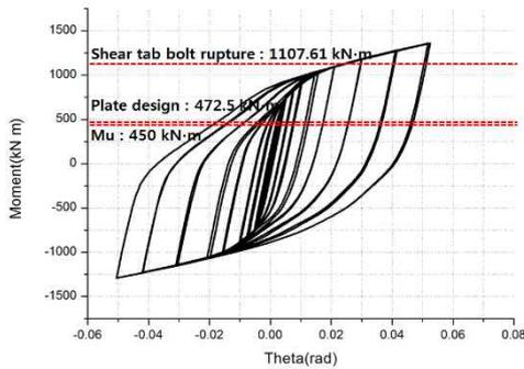
(b) Welded flange plate connection
