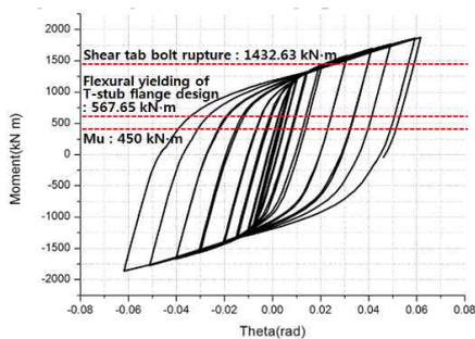
(d) High-strength bolted double split tee connection
