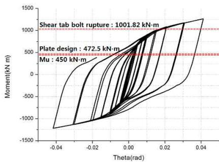
(c) High-strength bolted flange plate connection
